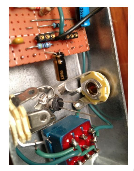
Loop the negative (shorter) LED lead around one end of the 4.7K resistor and solder them together.
