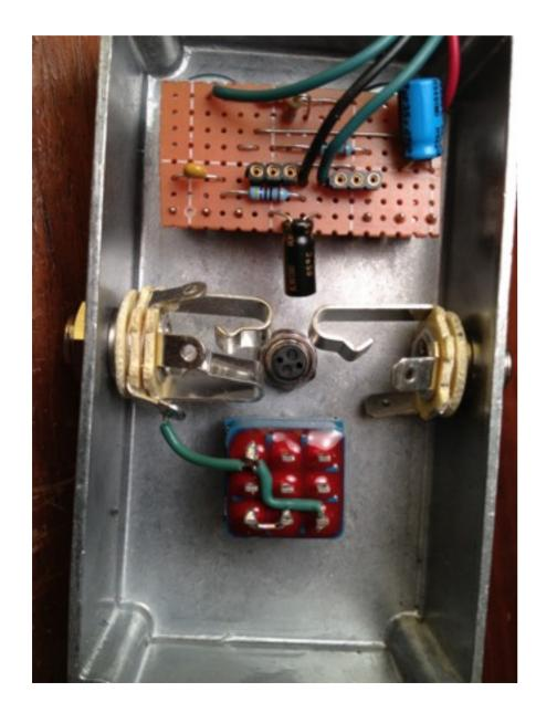
Solder a short length of wire between the output jack's outermost lug (the ones closest to the side of the box) and the center-left footswitch lug.
