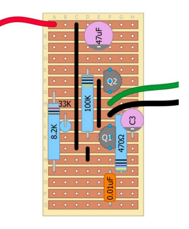
Cut a 4" piece of wire and solder it into row O at column A.
