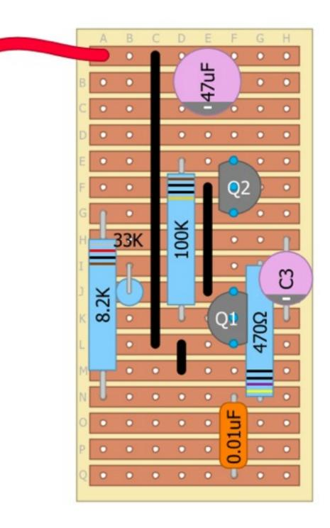
Cut a 4" piece of wire and solder it into row I at column F.
