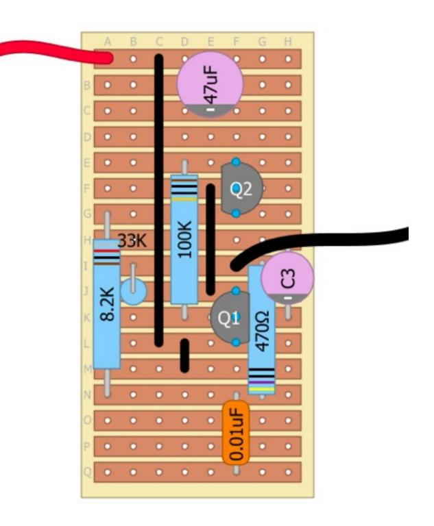
Cut a 4" piece of wire and solder into row H in column F.
