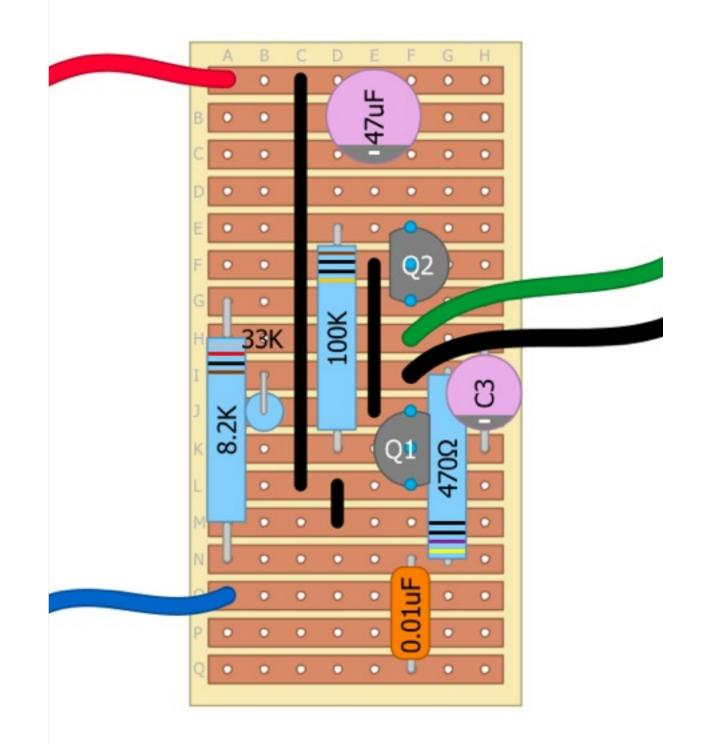
Solder the 1K pot to rows A, C, and E at column H. (If you use pots with lug-style connectors, solder three short lengths of wire into these holes, and then solder the other ends to the pot lugs.)
