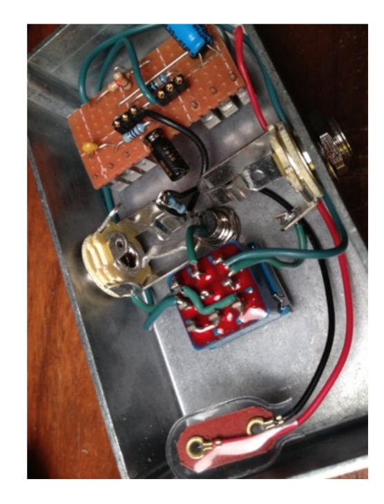
You can apply or bit of heat-shrink tubing to the LED solder junction to prevent it from shorting out against other connection, or just wrap the connections with electrical tape.
