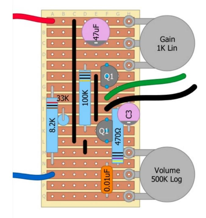
Here the wires are labeled. This is a PNP version that uses a positive ground.
