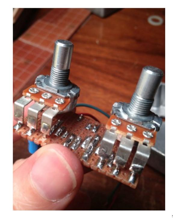
Mount the PCB board to the box. (If you're not using board-mounted pots, use double-sided adhesive tape to secure the board.) Attach the pots' screws, securing the board in place.
