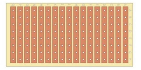
I like to cut the board across the holes, rather than trying to cut between the strips of copper.
