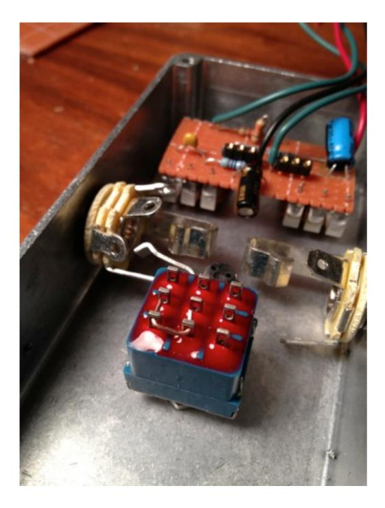
Run a short length of wire between the footswitch's upper-left and lower-right lugs. Solder it into the lower-right lug, but **don't solder it into the upper-left lug just yet.** Keep the insulated coating on this wire so the wire doesn't touch any lugs other than these two.
