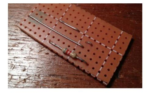
(I'll use this Fuzz Face schematic to illustrate the progress of our build, highlighting each component in red as we add it. Note that while this particular specifies 2N1305 transistors, I'm using AC-128s. Most PNP-style germanium transistor work fine, as do many silicon-type PNP-transistors.)
