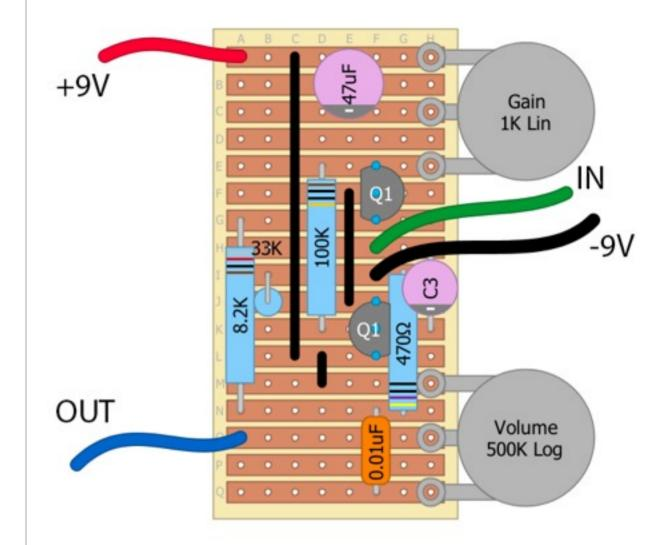
Here's my completed board. I used sockets for the transistors. I tested with two AC128 types. I'll need to cut down the leads before I box this up.
