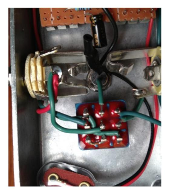
Solder the battery clip's red wire to the input jack's middle lug. (Middle, that is, relative to the side of the enclosure.)
