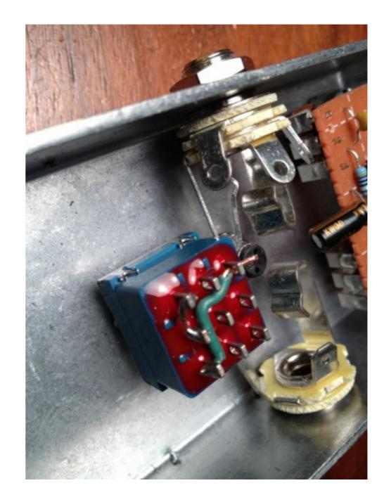
Solder a short length of wire to the input jack's outermost lug (the ones closest to the side of the box). Solder the other end to the upper-left lug, together with the wire previously placed there. (You don't necessarily need to thread both wires *through* the lug, so long as the two are securely soldered to this point.)
