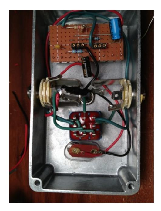
Insert the transistors, trimming their leads as necessary. (Your transistors may look different from these.)
