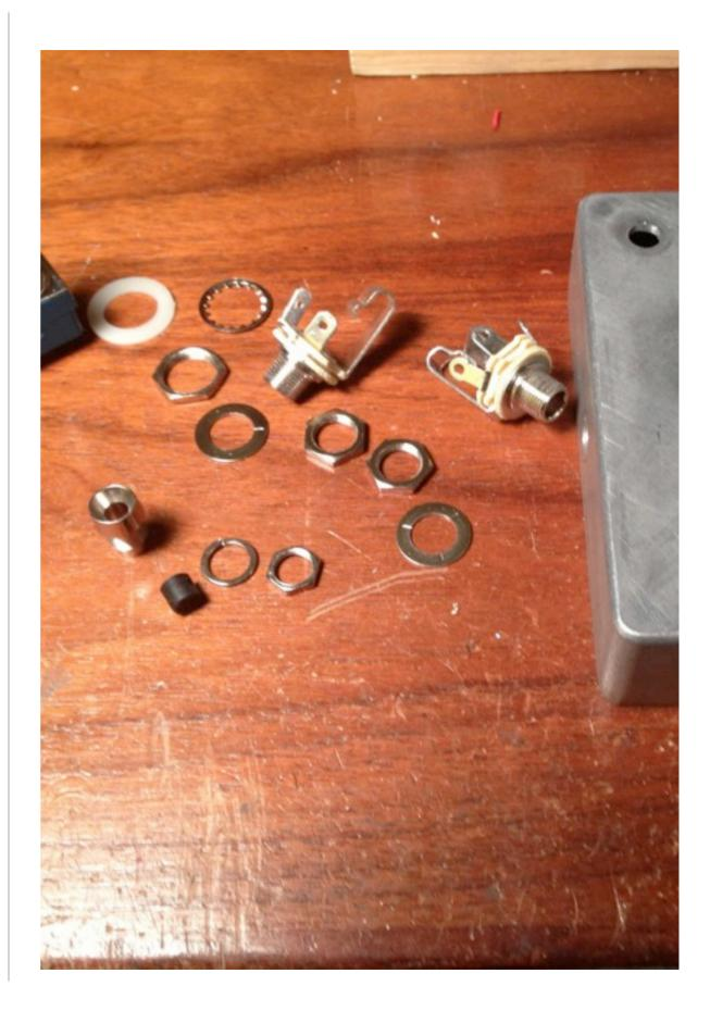
I drilled a blank box, and then mounted the switch, LED bezel, and input and output jacks. Here's what my box looks like.
