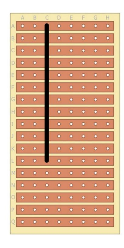
Cut a 1/2" length of wire and solder it between L and M on column D.
