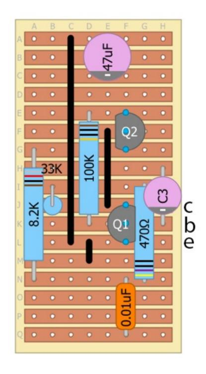
Cut a 4" piece of wire and solder to row A at column A.
