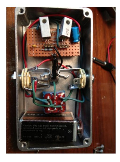
Gently bend the transistors and large capacitors so that they won't touch the back of the enclosure when you screw it in place. (Don't worry about the output jack's empty lug — the jack is grounded via contact with the enclosure.)
